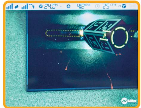
During a simulated weld sequence, visual graphical aids guide user to achieve adherence to parameters.
