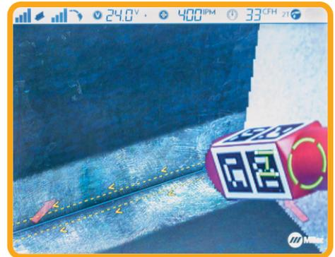
Actual proximity and interaction data is processed by the system via specially coded devices and coupons
